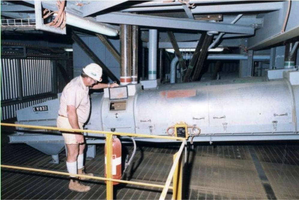
Figure B.4.: Enclosed drop-points on conveyor systems
