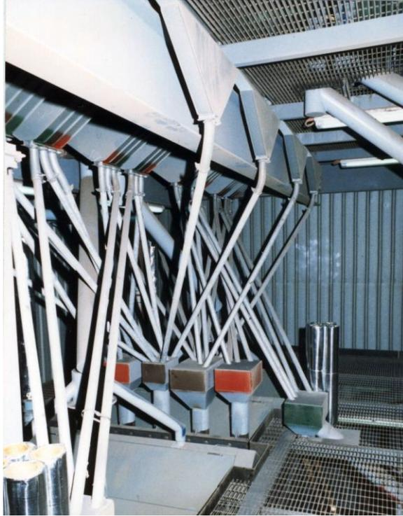
Figure B.8.: Test rig for determining optimum ventilation parameters – enclosed, ventilated drop box
