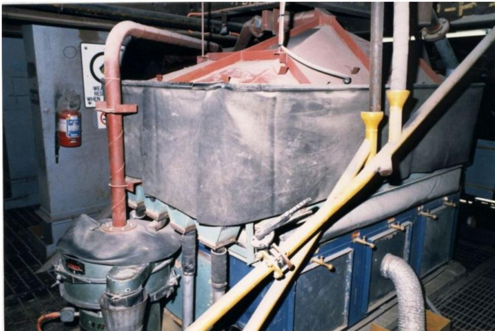
Figure B.7.: Feed distribution arrangement to HTRs – note enclosed feed hoppers, spillage collection hoppers and inspection doors
