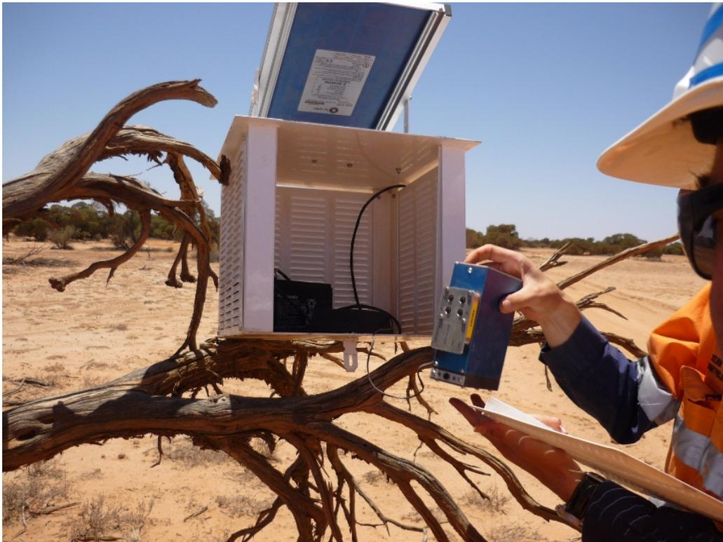
Solar/battery powered radon sampler
